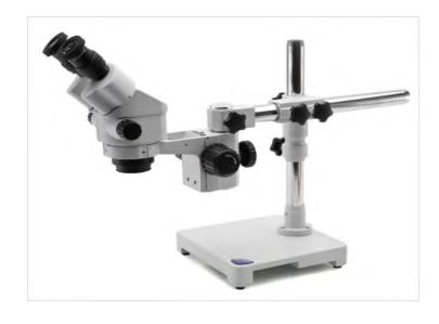
Binocular stereozoom microscope, 7x...45x, simple overhanging stand
